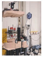
On the basis of the load case to be validated, we use CAE simulation to develop a suitable impactor. Working with with high-precision machinery, this is then produced in-house, in a suitable material and with the calculated weight.
